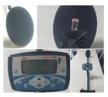
Lightly used: Minelab 705 gold detector, gold coil 18.75 Khz. Operates in three different frequencies depending on coil use
